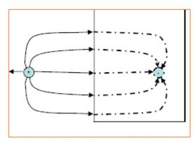
Figure 3. Charged particles are attracted to their mirror charge nearby conductors.
